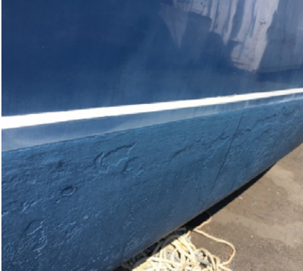
Photo above: Rough antifouling surface damages hull performance
